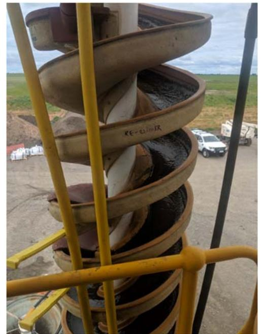
Figure 4: detail of the spiral separator module
