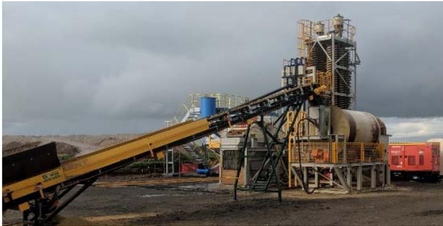
Figure 3: Avonbank Pilot Plant feed hopper conveying ore into the scrubber and trommel section of the MUP
