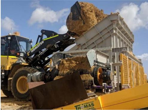
Figure 1: Avonbank Pilot Plant: MUP ore receipt via feed hopper
