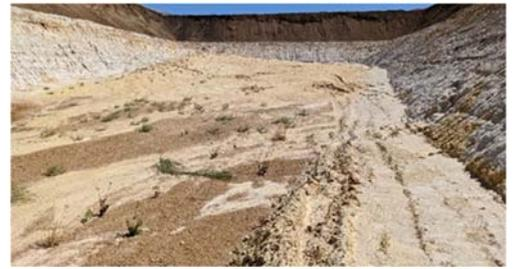
Figure 4: Avonbank Tailings placed into the test pit void, after wet gravity processing
