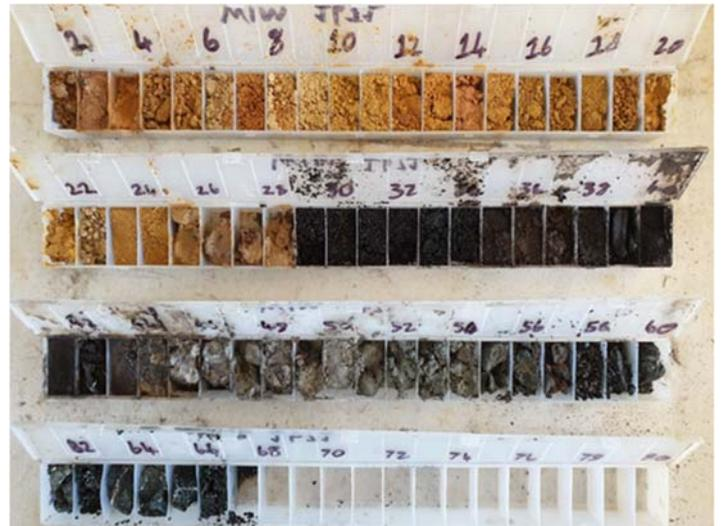
Figure 4: typical chip tray of drilling samples.
