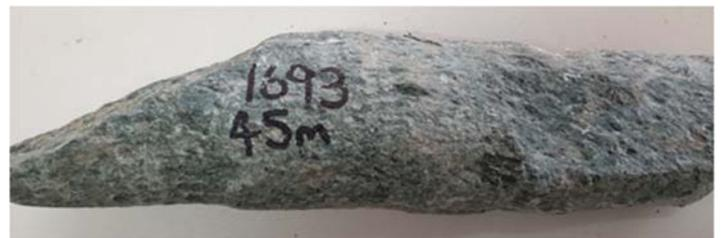
Figure 5: sample of drill core from hole WIM1693, 45m depth, Cambrian basement
